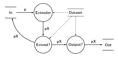
We can see that the different query extension processes do not share a dependency, except the dataset. Dataset itself is read-only in a given process, which means that we can use multiple extender processes. The same applies for extendable and output filter.
